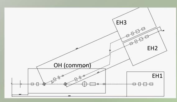
Source: two canted undulators to serve side and central branches Diamond splitters as monochromators for side branches DCM for the central branch Robotic sample changers
