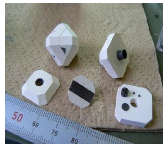
Kimberlite melt viscosity measurement by method sinking spheres at 6 GPa and 1200-1600 ° C
